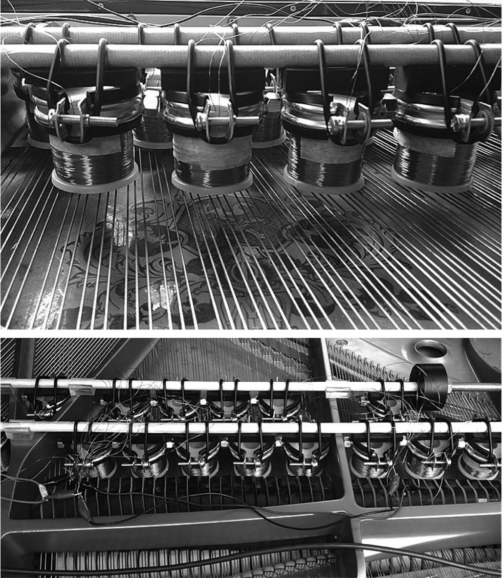
**Figure 3:** Actuator setup offered by the write, on a concert piano. Sixteen solenoids are placed on piano strings.
