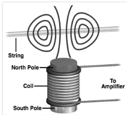
**Figure 2:** Typical electric guitar pick-up – the red edge is the north pole of the magnet sitting inside the coil, blue lines indicate the magnetic field. The movement of the string causes a change in the magnetic field that creates voltage in the coil [12].
